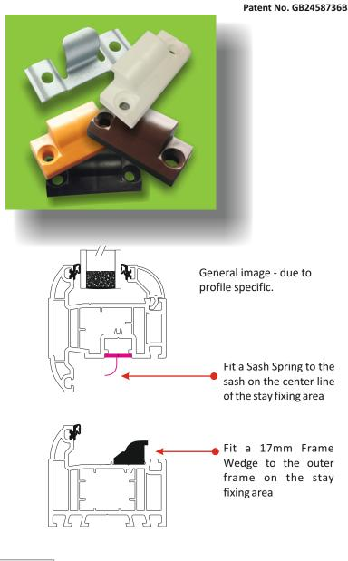
Fit a Sash Spring to the sash on the center line
